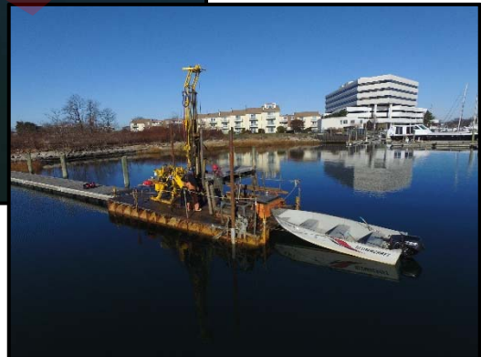
Soil boring being completed at West Beach boat ramp, looking north, photo taken by RTG on December 19, 2018
